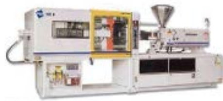
• Injection Molding Machine Dong HYDATics Pro150 (Nozzle spec, 120 ton)
