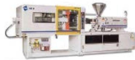
• Injection Molding Machine Dong HYDATics Pro150 (150ton)
