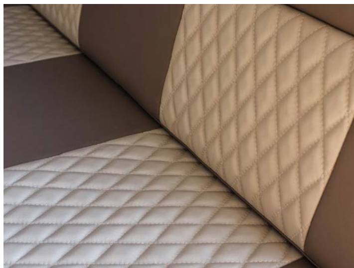
Diamond straight stitching pattern (dual hides)
