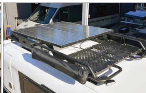
Rear platform for bulky light storage items
