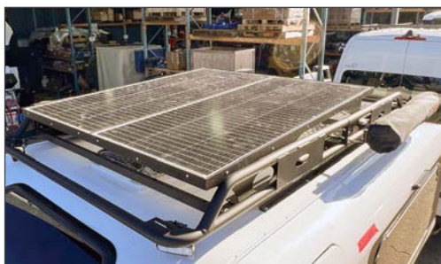
Fly over solar panels for 400W capacity
