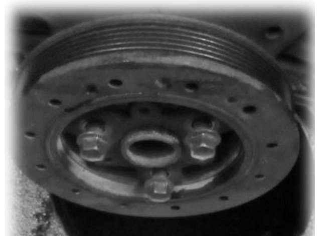
Figure 6 – Crank pulley bolts being removed
