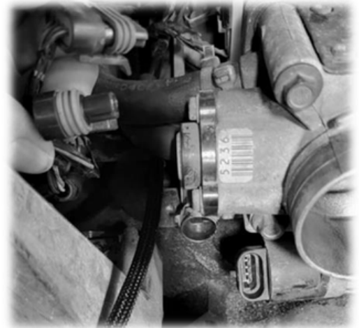
IAC and TPS sensors unhooked
