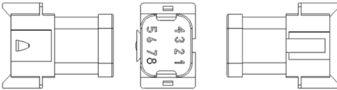
Connects to programming connector on main harness
