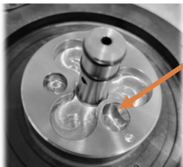
Figure 3 – Pin drive spindle. Has locating hole for cam dowel pin. This drive hole is oval in shape
