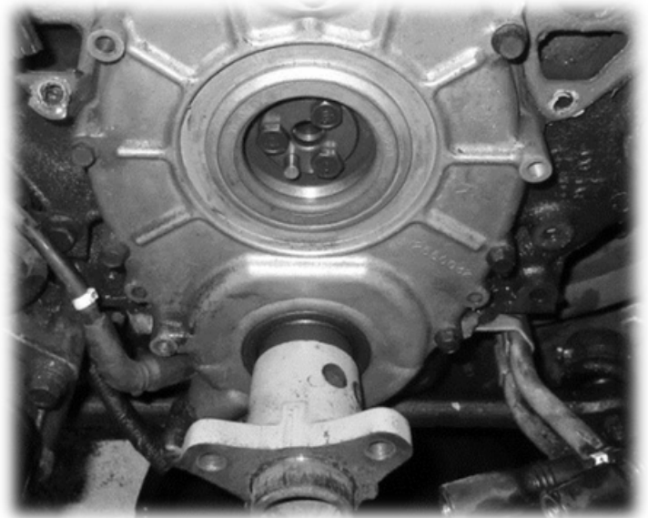
Figure 9 – Optispark Distributor removed. Late model type shown.
