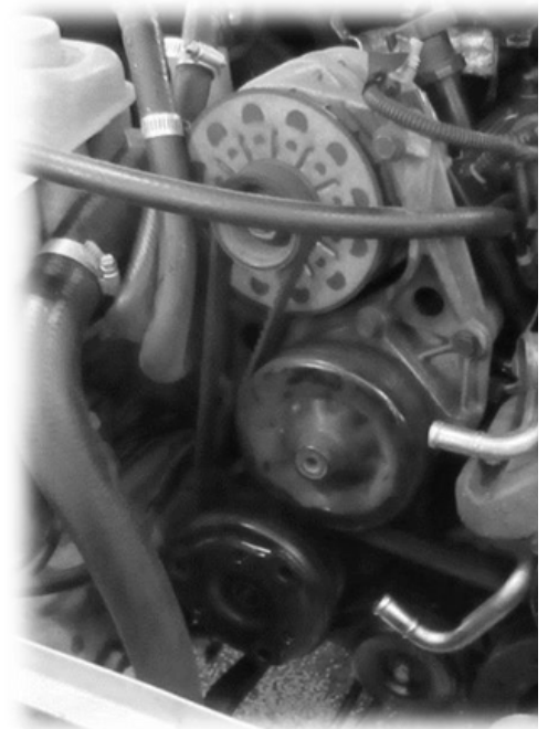
Figure 5 – Heater core hoses removed
