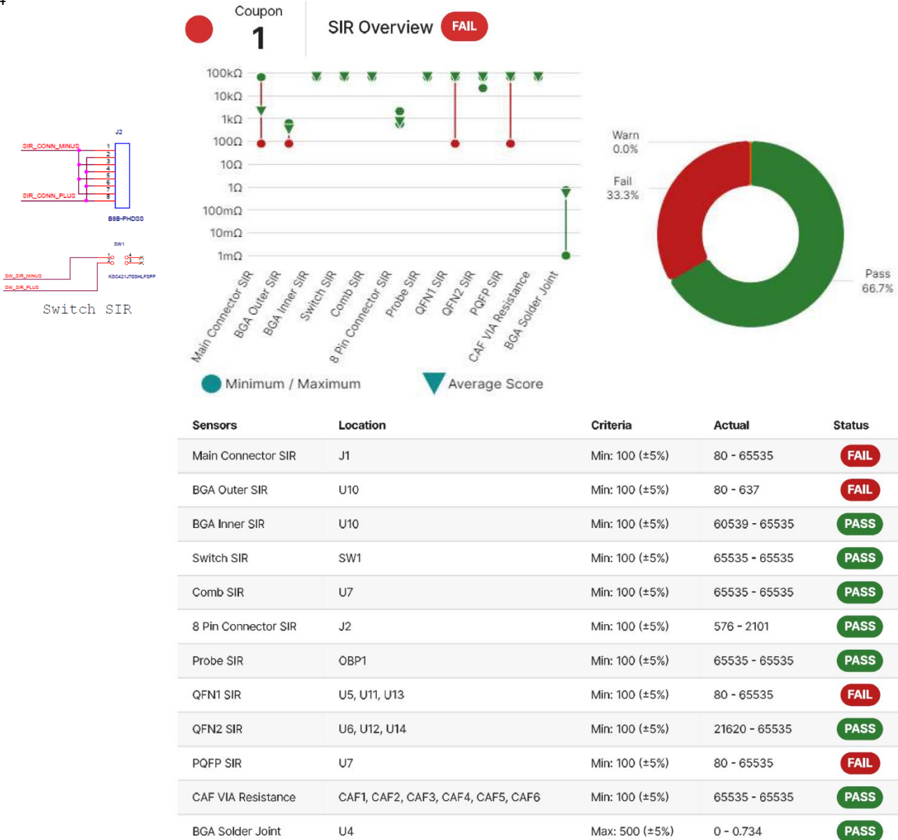
305 306 Figure 17: SIR Data Findings for Each Component on the Test Board 307 308 309 310
