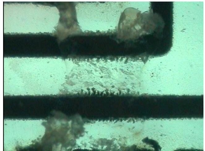
Figure 2: Active Flux Residue under the BTC
