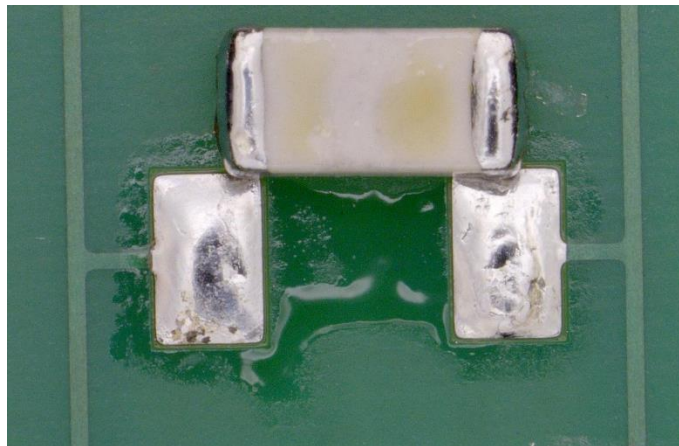
Figure 3: Desoldering Components can cause flux residue to flow under the component termination
