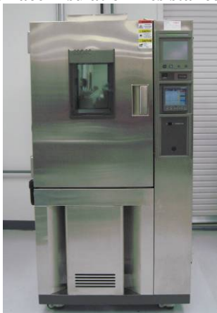
Atmospheric Control Chamber Element of an SIR System
