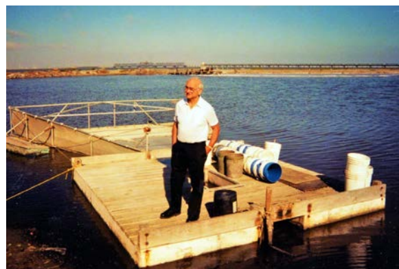
The author standing on brine shrimp ( artemia ) collecting boat in San Francisco salt ponds. The boom in the front section is wide at the mouth to allow the ribbons of shrimp to funnel into a small opening in the rear section, where workers with nets can capture the shrimp and place them in buckets to be frozen into packages.
