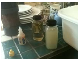
Figure 14: Testing tapwater. The bottle on the left is distilled water (the control) with reagent. The bottle on the right is tapwater with calcium and magnesium precipitating out after reaction with the reagent. Hardness measured 16 grains per gallon.
