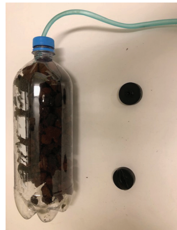
DIY version: Seltzer bottle, lava rock, 2 magnets used to attach to side of tank
