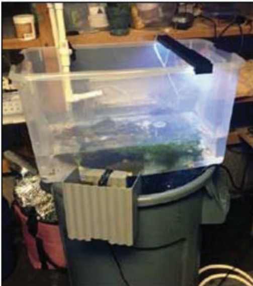
Water in the Brute sump passes through sponge filters, biomed, and an HOB filter.
