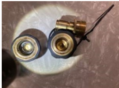
Worn-out Quick-connect fitting on Left
