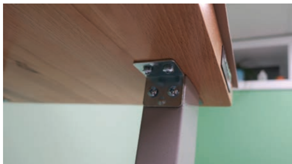
Two brackets are attached to the bottom of the work bench by four screws per bracket. On the other side of the leg, hidden from view, is an identical bracket. Eight screws attach each leg to the bottom of the bench top. All four legs use a total of thirty-two screws.
