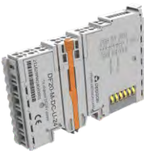
Voltage distribution module, 16 channel 24VDC
