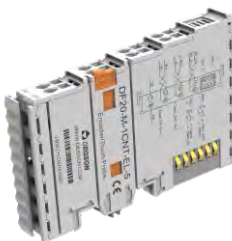
Encoder input module, 1 port,5V
