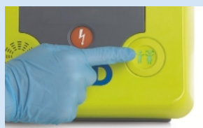
Child button will illuminate when pediatric pad is attached.
