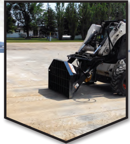
ADJUSTABLE FLOW CONTROL TO SPREAD OVER DISTANCES FROM 4' TO 35'
