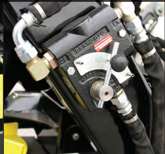
ADJUSTABLE FLOW CONTROL TO SPREAD OVER DISTANCES FROM 4' TO 35'
