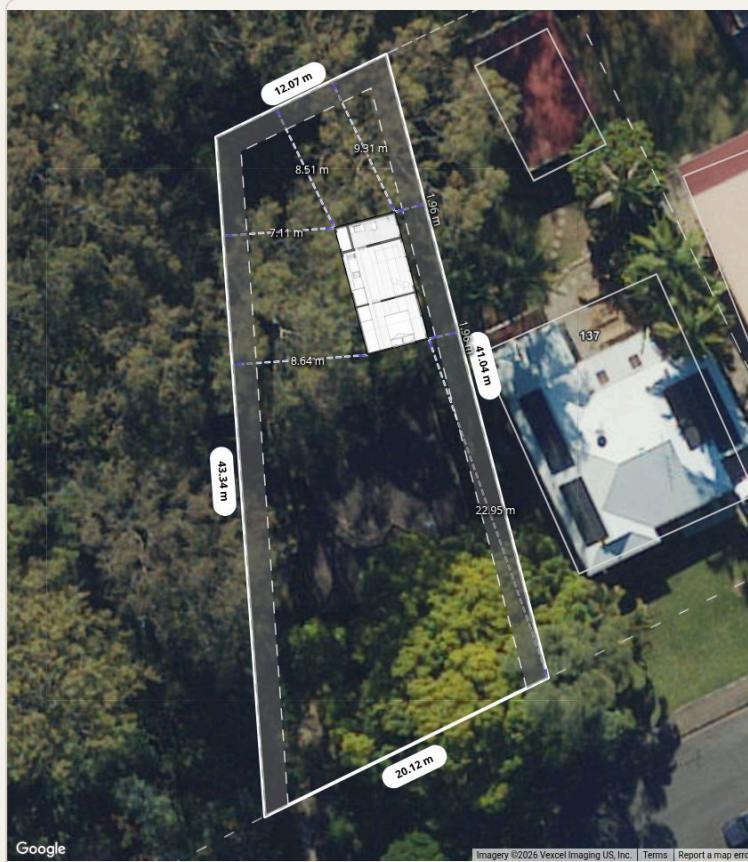
Proposed siting with boundary setback dimensions. Not to scale (Canibuild).
