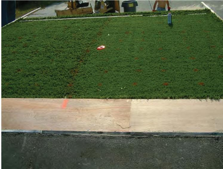
FIGURE C-18. TEST 2b—2.5-INCH FIBER TEST PLOT (SECOND INSTALLATION)
