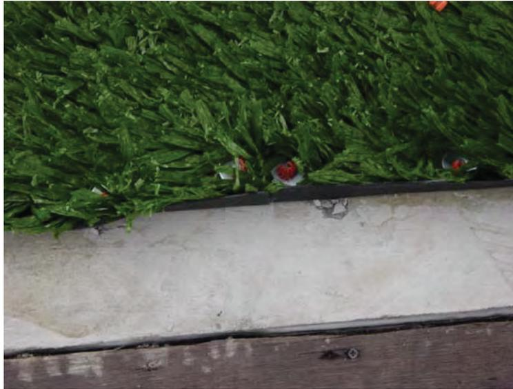
FIGURE C-41. THE 2.0-INCH FIBER WITH RUBBER HEADER
